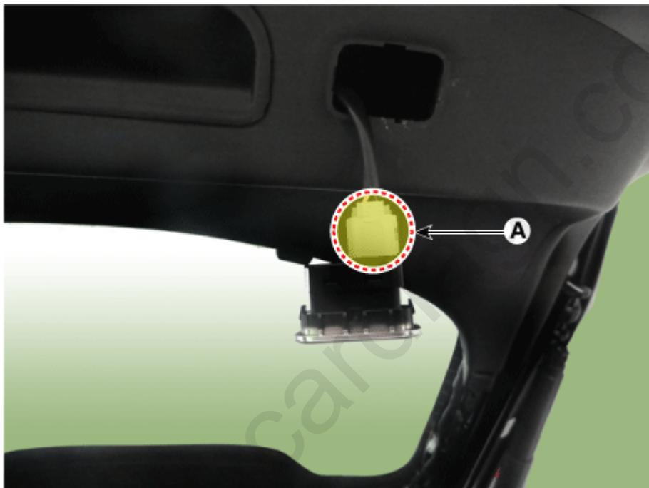
6. Remove the tailgate trim (A) after loosening the mounting screws.
