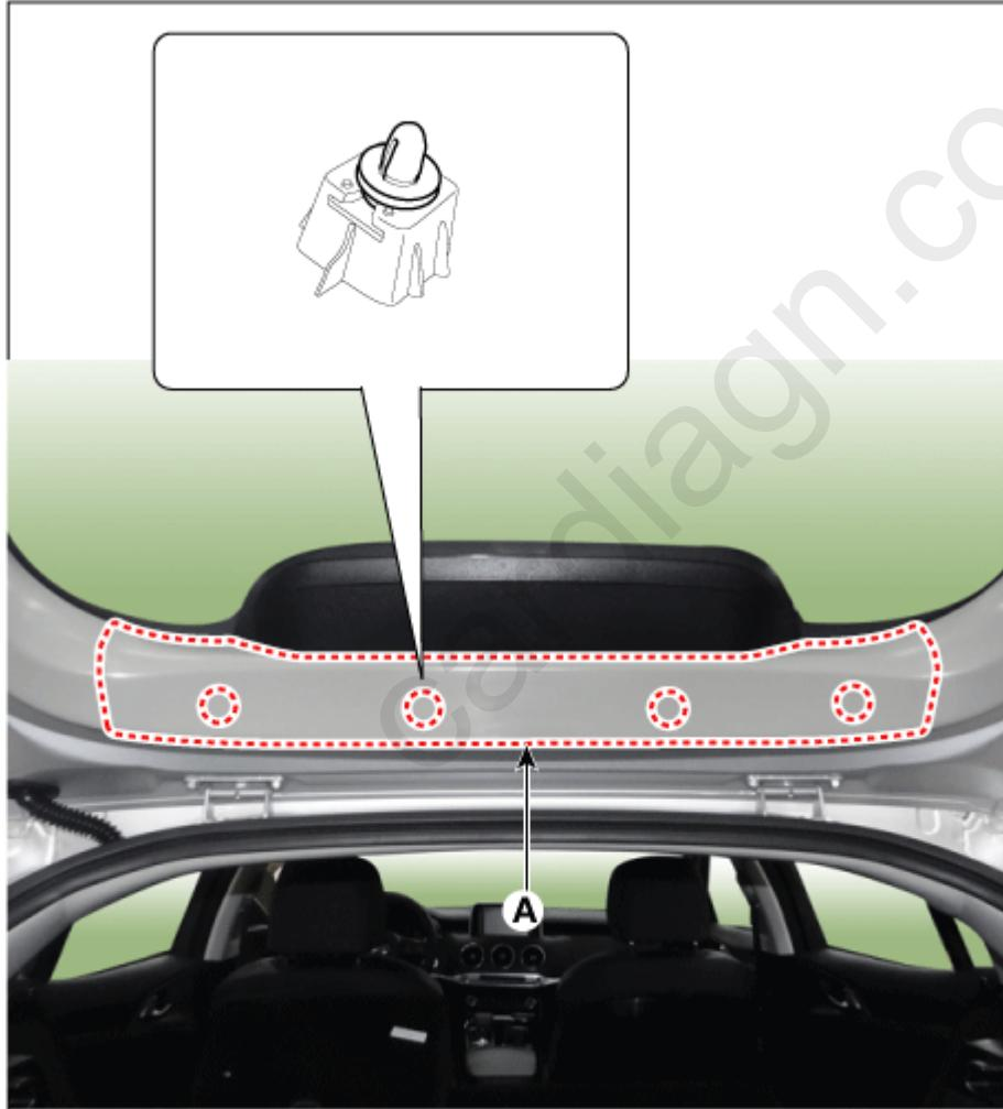
2. Remove the tailgate side trim (A) after loosening the mounting screw.
