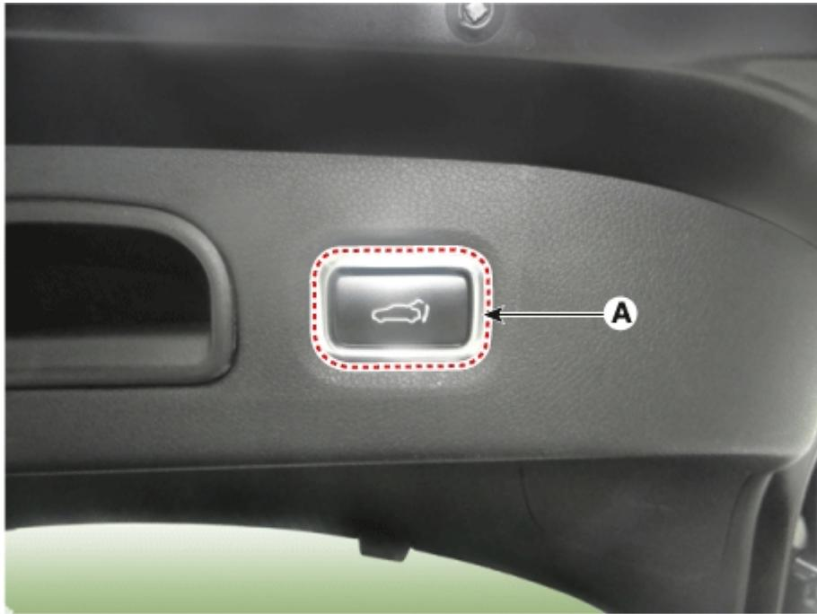
5. Remove the smart tailgate inner switch after disconnecting the connector (A).
